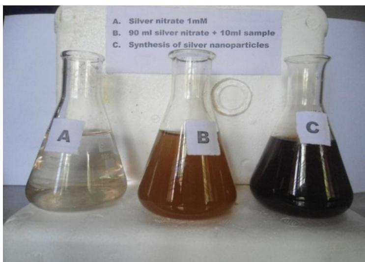
Figure 1. A. Silver nitrate 1mM, B. 90 ml silver nitrate+10ml sample and C. Synthesized silver nanoparticles from broiler chicken faecal excreta.
